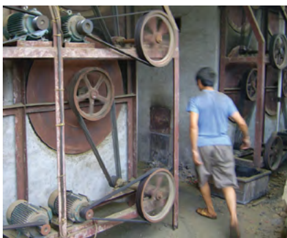
Unguarded machine: bad practice demonstrated in the toolkit
